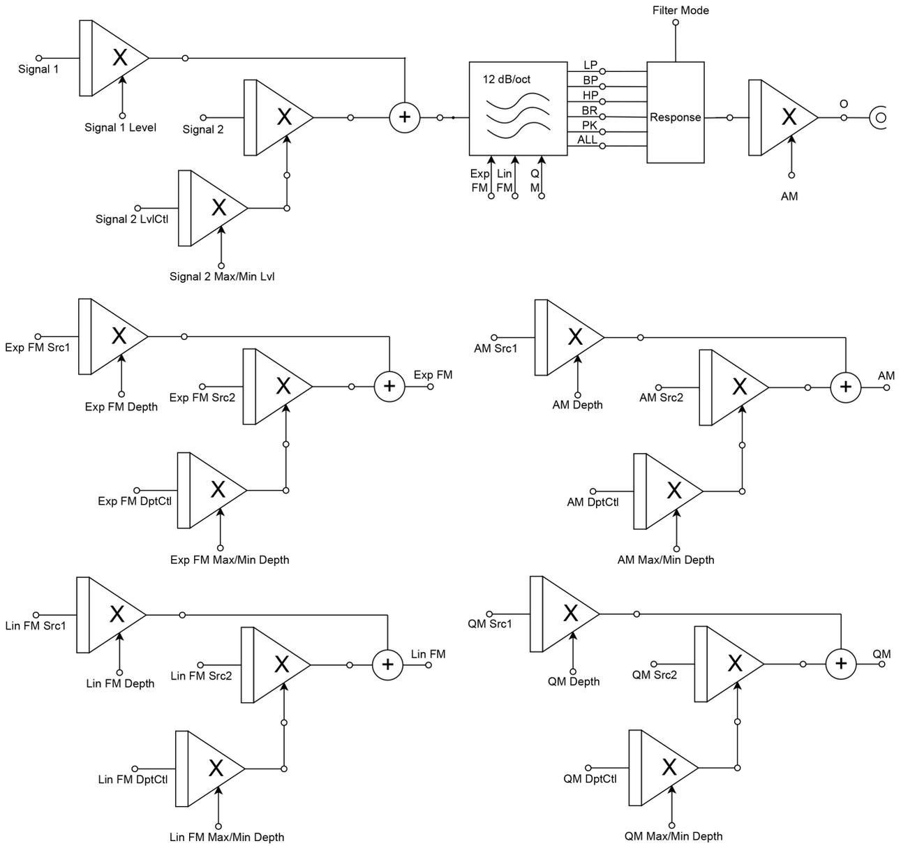
Each filter has 2 signal inputs.
