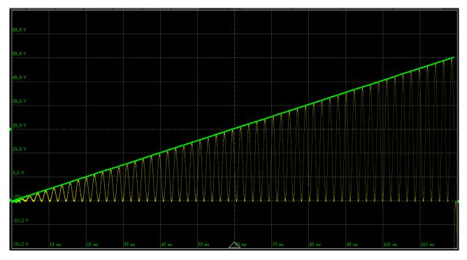
AM Max Depth = 1.000, Min Depth = 0.000With the bias pot at minimum there is no AM, with the bias pot at maximum, there is max. AM.
