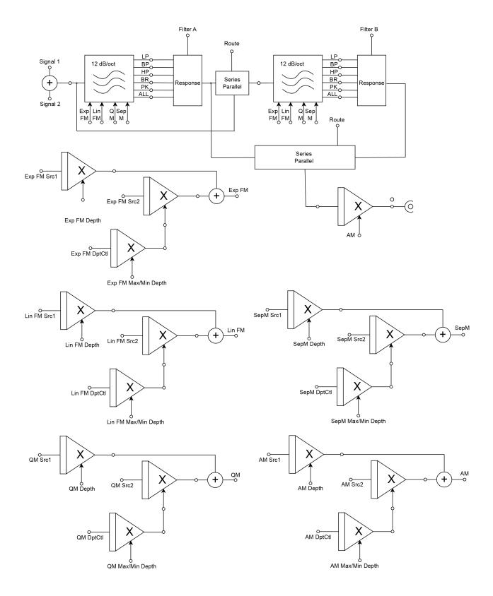
Each filter has 2 signal inputs.
