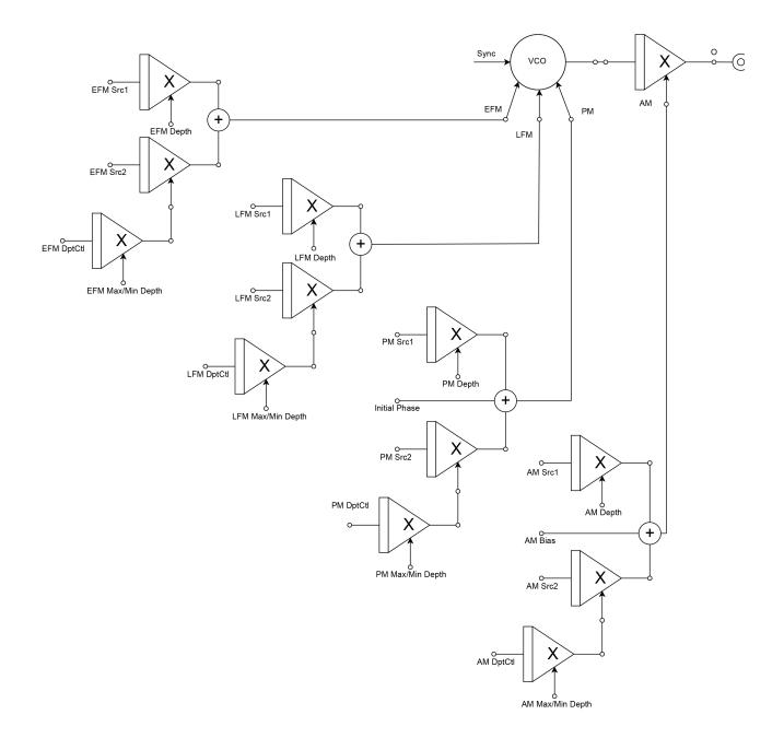
Each oscillator has 4 analog control inputs : E(xponential) FM, L(inear) FM, PM and AM, and 1 digital control input : Sync.
