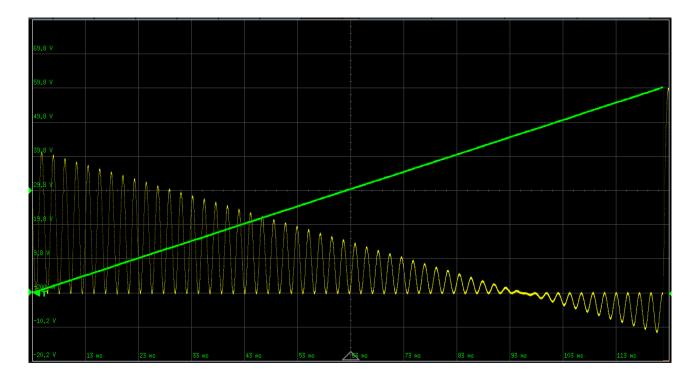
AM Max Depth = -0.200, Min Depth = 0.700Any combination of Max and Min, positive or negative is possible.
